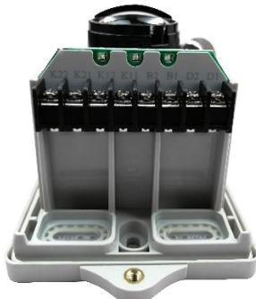
Fig. 11a – Wiring terminals
